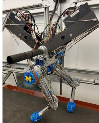
Figure 1: This work investigates the difference between forward and backwards gait on the robot *RAMone*. It was built at the University of Michigan as a testbed for studying efficient gait. The robot is based on the *ScarLETH* leg design [4], and is mounted on a two dimensional gantry which restricts its motion to the sagittal plane.
