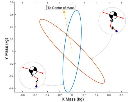
Figure 3: Contact space mass ellipse for a likely contact configuration in knee forward and knee backward cases. We see a larger apparent mass in the direction of the center of mass in the knee forward case. Since it is desirable for the contact impulse to lie in this direction, this points to a larger collision loss with the knee forward.
