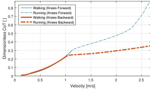
Figure 2: Energetic cost of transport across a range of speeds for both forward knee and backward knee walking. We see that the walking cost of transport coincides between the two cases, while the backwards knee running gait is significantly more efficient than the forward knee gait.
