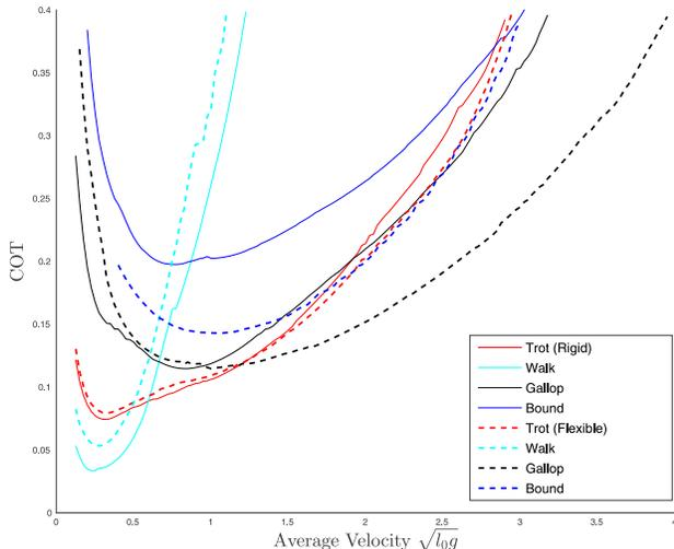
Figure 2: The combined energy cost landscapes of both the rigid model and flexible model for different gaits and speeds. The combined curves show a distinct energetic benefit for galloping with the flexible model at higher speeds.
