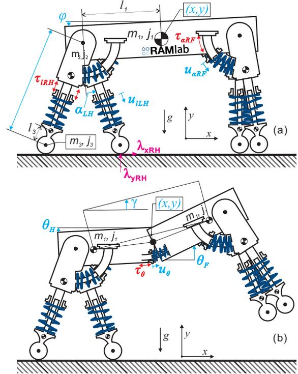
Figure 1: In this work we compare the energetically optimal motion of a robotic quadrupedal model with a rigid spine (a) to a model with an articulated spine (b) to see the energetic effects of a flexible spine.
