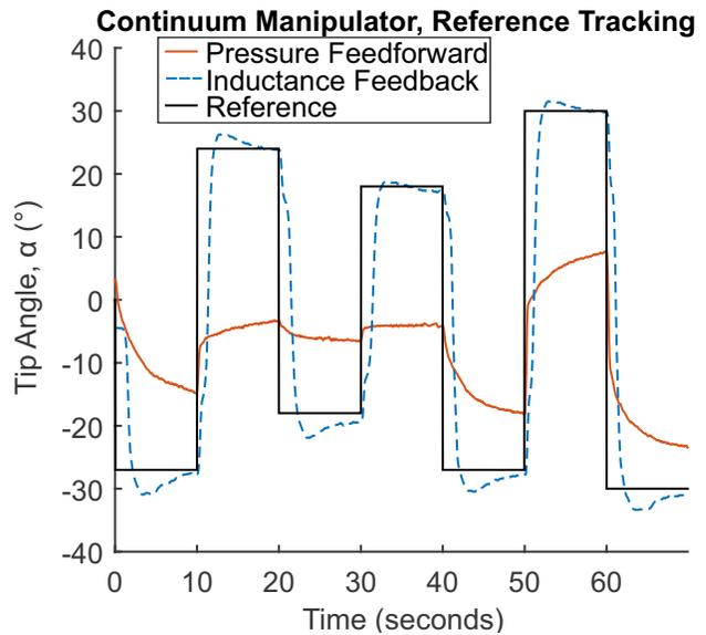
Fig. 4. Using the inductance as feedback to control the tip angle of the Smart Braid McKibben muscle continuum manipulator results in an average steady-state error of  $1.25^\circ$  (blue line, partial test shown). This is a dramatic improvement over the performance of an open-loop controller that relies only on the pressure (red line). Adapted from [4].
