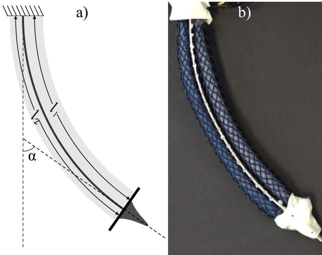
Fig. 3. By attaching two McKibben muscles to a flexible “spine,” a planar one-degree-of-freedom continuum manipulator is made. The conductive wires (black) form “Smart Braid” circuits with inductance values that increases as their corresponding actuator contracts. Adapted from [4].
