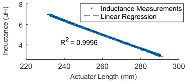
Fig. 2. A contracting fiber-reinforced actuator can be outfitted with a “Smart Braid” that measures the contraction via a linear inductance response. The braid is made from off-the-shelf wires that provide both reinforcement and sensing to the actuator. Sensors such as these can be used to control soft robotic systems driven by fiber-reinforced actuators [4]. Adapted from [1].
