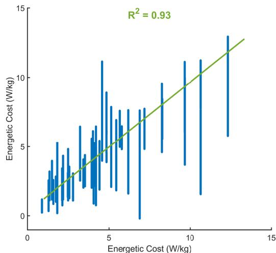
Fig. 4. Regression model containing data from all subjects and all ambulation tasks. We trained this model using both physiological signals (heart rate, electrodermal activity, and skin temperature), and mechanical signals (linear envelope EMG and accelerometer magnitudes, both processed with a 10s sliding window average). The coefficient of determination was  $R^2=0.93$ .
