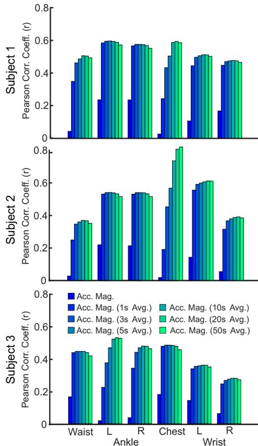
Fig. 2. Correlations between accelerometer magnitudes (Acc. Mag.) and ground truth energetic cost for accelerometers fixed to the waist, chest, and left (L) and right (R) ankles and wrists of each subject. Accelerometer magnitudes were processed using a sliding window average. The effect of different window lengths on correlation is shown. Window lengths increase from left (dark blue) to right (light green), and correspond to no average, and 1, 3, 5, 10, 20, 50 second averages, respectively.
