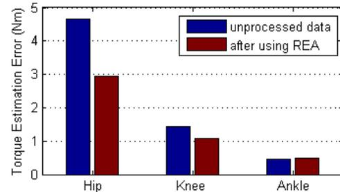
Figure 2. Average torque estimation error for hip, knee, and ankle flexion and extension with 12mm Noise SD
